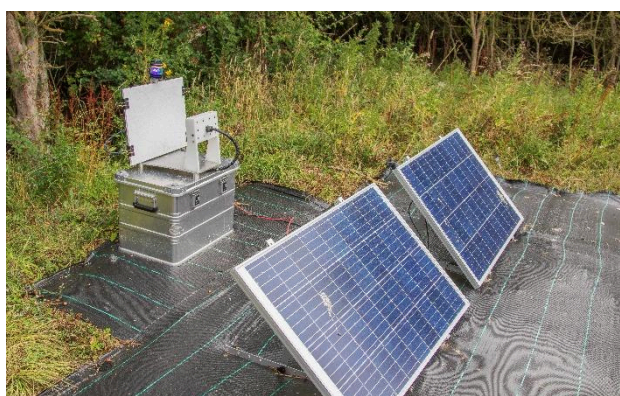
Figure 22: MAMBO research equipment for automated surveying and identification of moth species. (Photos: H. Wilkinson)
