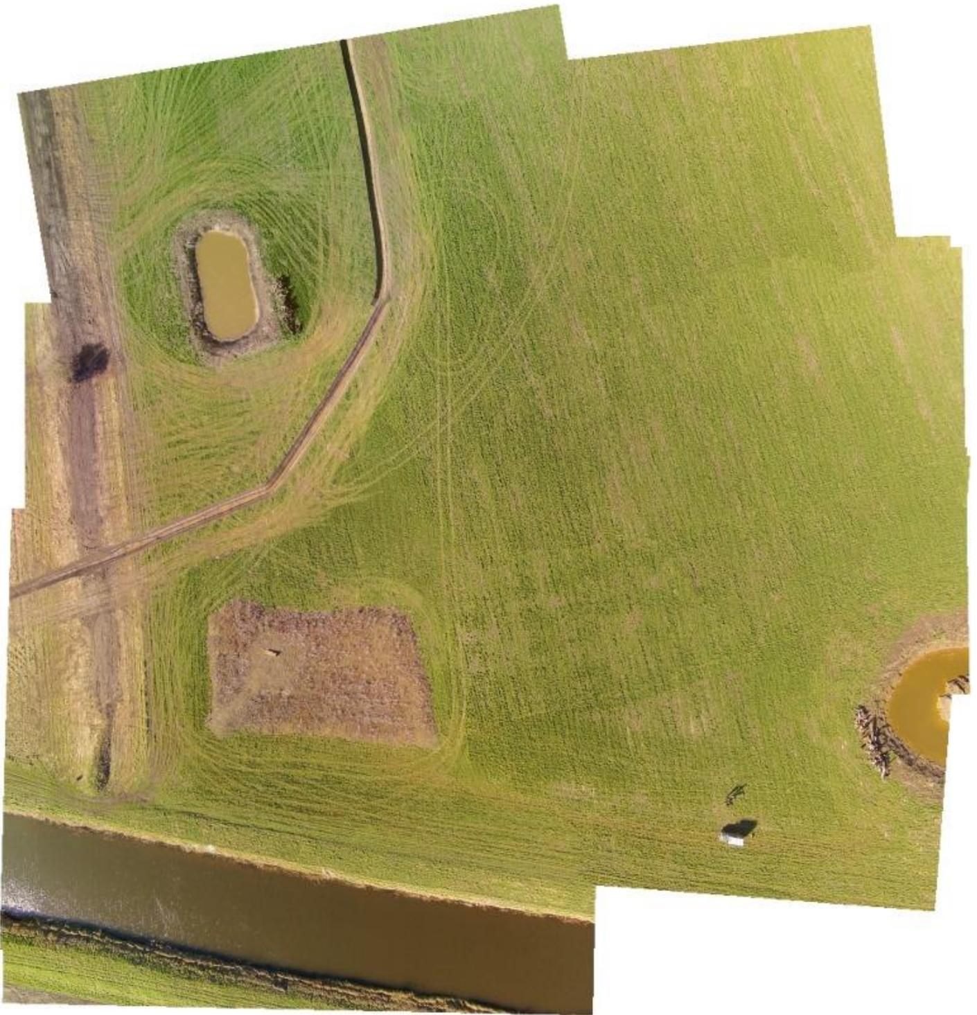
**Figure 4 Tiled image of Engine Farm showing earth mound, new ditch, new ponds and MLC drainage channel**
