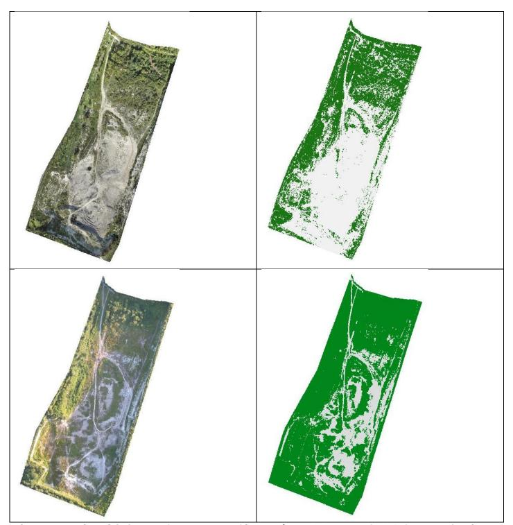
Figure 1 East pit aerial photo and remote sensed images from 2010 (top and 2016 (bottom) showing bare chalk in light grey and vegetation in green.
